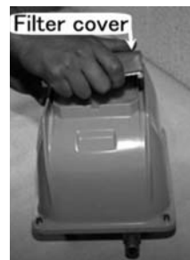
2. Remove the filter cover.
