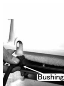
4. Pull out the bushing
