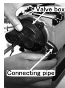
11. Pull out the connecting pipe and remove the valve box of one side.
