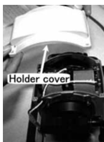
7. Remove the holder cover.
