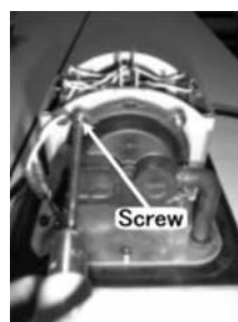
9. Undo the screws
