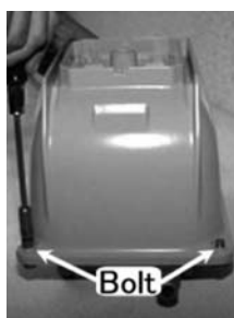
1. Undo the four corner bolts.
