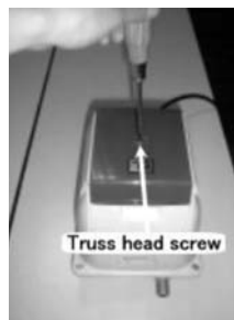
1. Undo the truss head screw.
