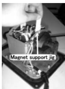
8. Insert the magnet support jig in four corners between magnet and core.
